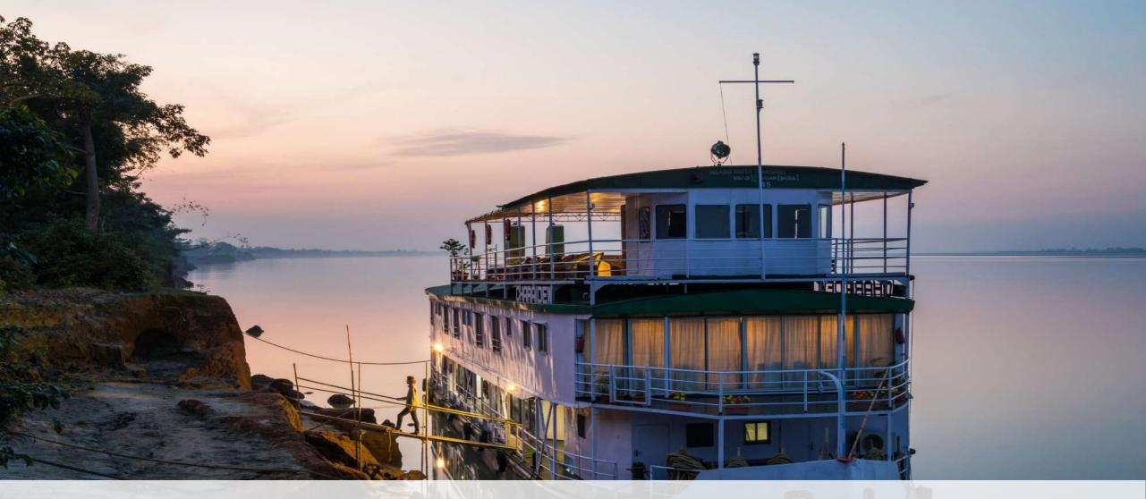
**ABN Charaidew (comfort)** is a 38m-long, twin-engined, steel hulled passenger boat. She was completely stripped down and rebuilt by Assam Bengal Navigation in 2003 to provide 10 twin-bedded and 2 double-bedded cabins with en-suite bathroom.
